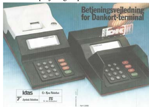
Fig. 2. The Dankort terminal. To the left the shop cashier's terminal, where she entered the amount and printed the receipt. To the right the customer terminal with card reader and key-board for the PIN-code.
