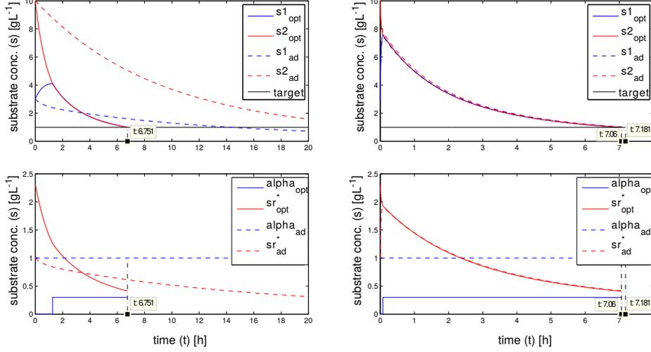
FIGURE 5. Trajectories and controls generated by the two-pumps and one-pump optimal feedback, for  $r = 0.3$ ,  $\underline{s} = 1[\text{g}\cdot\text{L}^{-1}]$  and  $s(0) = (3, 10)[\text{g}\cdot\text{L}^{-1}]$ . On the left  $d = 0.1[\text{h}^{-1}]$ , and on the right  $d = 10[\text{h}^{-1}]$ .
