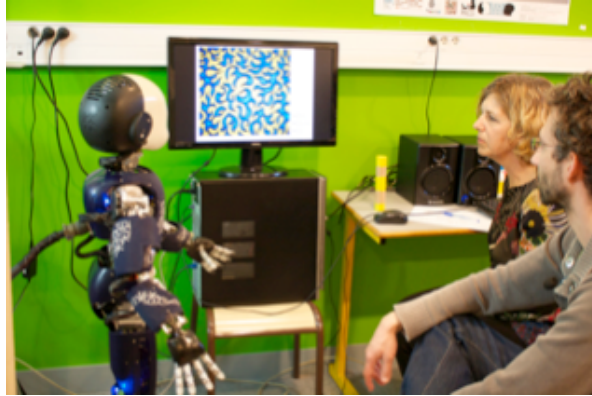
Figure 2 - Functional task, evaluation of images. The robot is gazing at the screen where the image to evaluate is shown.
