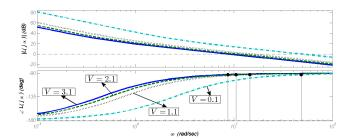
Fig. 8. Bode plot for the the loop transfer function  ${\cal L}$  with different values of V
