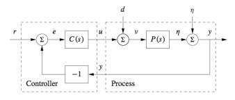
Fig. 1. Block diagram of a linear feedback loop
