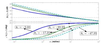
Fig. 9. Bode plot for the the loop transfer function L with different values of  $k_1$
