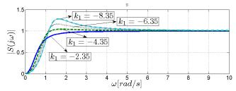
Fig. 6. Gain curve of the sensitivity function S for the second-order plant
