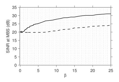
Fig. 4: The SINR received at the MBS against the parameter  $\beta$  after introducing the binary variable  $\delta$  in the utility functions
