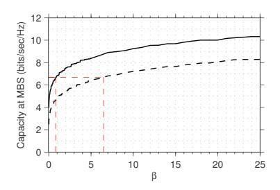
Fig. 3: The normalized capacity for the MBS against the parameter  $\beta$  for four different network topologies. The dashed red lines indicate the values corresponding to the critical SINR value of 20 dB at the MBS.
