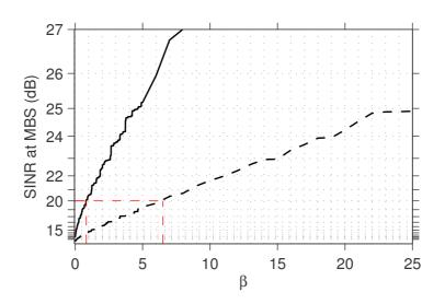
Fig. 2: The SINR received at the MBS (linear scale) against the parameter  $\beta$  for two different random topologies. The target SINR at the MBS ( $\gamma_{M_{target}}$ ), i.e., the critical point, is set to 20 dB.
