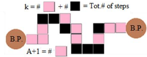
Figure 8: 2D 4-connected path showing the axonal trajectory until the formation of a branching point (3D not shown for simplicity). Pink pixels occur with a probability p , decreasing the growing rate. When the number of pink pixels equals A+1 , v_i=0 and a new branching point appears.
