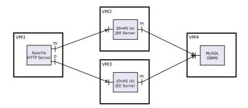
Figure 1. A Three-tier Web Application Model
