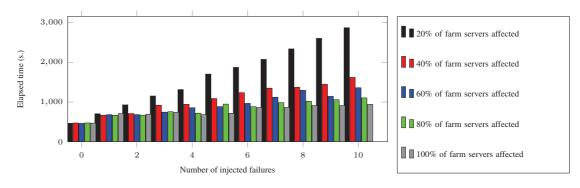
Figure 8. Time to Deploy a Three-tier Web Application (Farm of Servers) with VAMP while Injecting Failures
