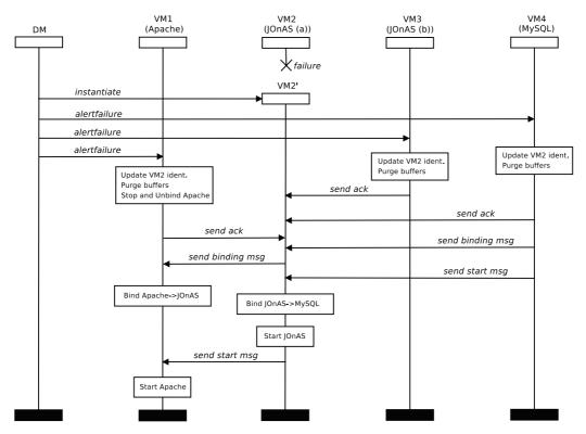
Figure 6. Web Application Failure Scenario
