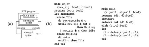
Fig. 1. Discrete control: (a) control model; (b) controlled automaton example.
