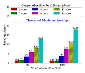
Fig. 2. Parallelization speedup factors for different job sizes and cores.
