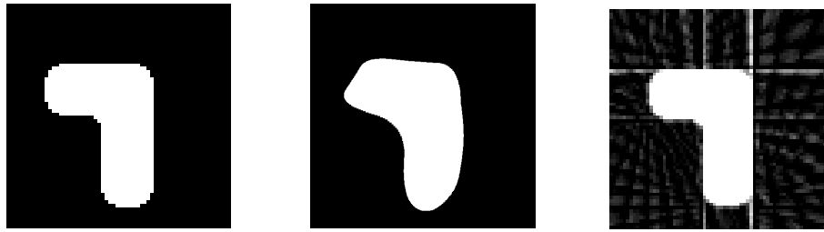
Fig. 6. Left: Original \Omega_1 . Center: NURBS-MCMC reconstruction. Right: FBP reconstruction. Both are using error 0.1%.
