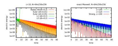
FIGURE 1. The Landau damping problem for a number of different second order L-stable schemes. The time step size is indicated in paranthesis. The analytically derived decay rate is shown as a black line.
