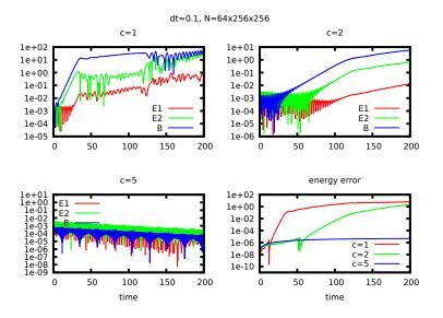
FIGURE 7. Fully relativistic case (Weibel problem): time evolution of the most unstable mode (k = 1.25) of the magnetic and the two electric fields obtained by AP-VM (for c = 1, 2, 5). Bottom right: time evolution of the energy error for c = 1, 2, 5.
