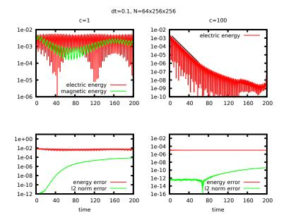
FIGURE 6. Fully relativistic case (Landau problem). Top: time evolution of the electric and magnetic energy obtained by AP-VM (for  $c = 1, 10^2$ ). Bottom: time evolution of the energy error and  $L^2$  norm (for  $c = 1, 10^2$ ). The analytic decay rate (-0.0661) for the Vlasov– Poisson Landau damping is shown as a black line.
