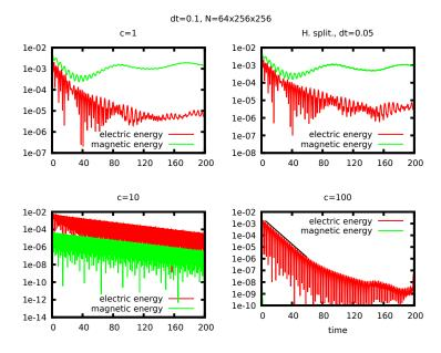
FIGURE 2. Semi-relativistic case (Landau problem): time evolution of the electric and magnetic energy obtained by AP-VM (for  $c = 1, 10, 10^2$ ) and H-split (c = 1).
