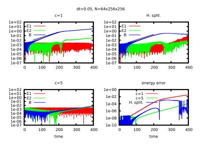
FIGURE 4. Semi-relativistic case (Weibel problem): time evolution of the most unstable mode (k = 1.25) of the magnetic and the two electric fields. Top left: c = 1, AP-VM. Top right: c = 1, H-split. Bottom left: c = 5, AP-VM. Bottom right: time evolution of the energy error for AP-VM (c = 1, 5) and for H-split (c = 1).
