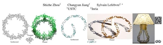
**Figure 1:** We use vector shapes as inputs to synthesize patterns along curves. The resulting patterns have a constrained topology allowing them to be 3D printed as a single piece. Left: Pattern along a circle and its printout. After printing, the pattern is a single connected object. Middle: Pattern along a curve and its printout. Right: A printed lamp modeled with our system, the shade and the foot are synthesized.
