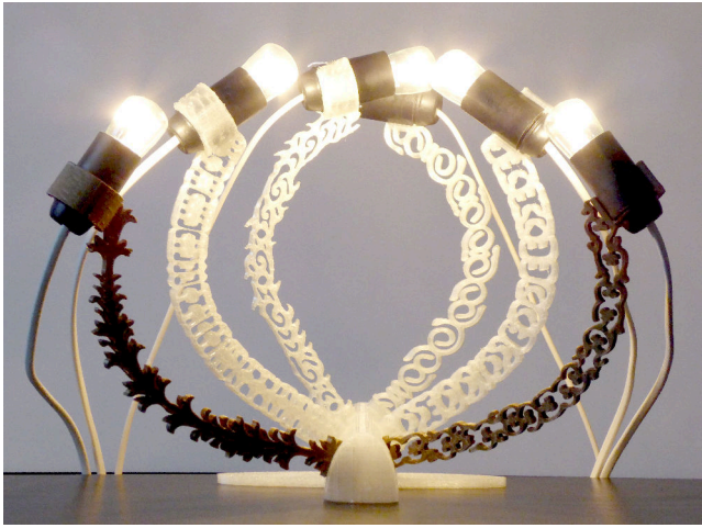
Figure 13: A lamp made of six curves synthesized with different patterns. Printed on an Ultimaker 2 (PLA plastic filament).
