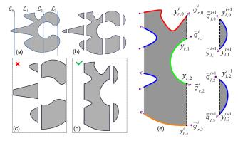
**Figure 3:** (a,b) Building pieces from an input exemplar. (c,d) Our algorithm only considers matching two pieces with the same number of portals (split lines marked by black dash lines in (e)).
