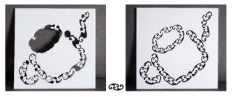
**Figure 24:** Printed objects. Left: Pattern synthesized and carved out of a plate. Without hole control several disconnected parts fell. Right: Pattern without holes synthesized from the same exemplar.
