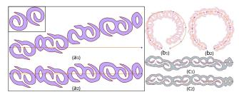
**Figure 8:** Results with  $(a_2, b_2, c_2)$  and without  $(a_1, b_1, c_1)$  global band fairing. The band fairing step avoids the result to drift away from the curve skeleton, and ensures a globally smooth appearance.
