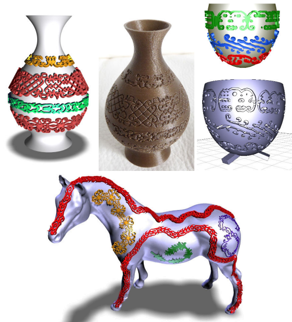
Figure 23: Applying our method on surface to decorate surface with synthesized patterns. The vase is 3D printed after embossing the synthesized patterns onto the initial model. The egg stand is obtained by carving the patterns out of a shell. Since the patterns have no holes, the result remains simply connected.
