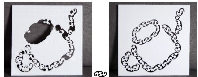
Figure 24: Printed objects. Left: Pattern synthesized and carved out of a plate. Without hole control several disconnected parts fell. Right: Pattern without holes synthesized from the same exemplar.
