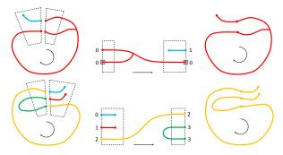
**Figure 6:** Synthesizing along a closed curve does not guarantee a closed pattern. Top: When joining the first and last piece, a closed loop is formed thanks to component ID 0 which has connected portals across the entire pattern (small black box). Bottom: When joining the first and last piece, only component ID 2 is connected from the start to the end. The final pattern has a single connected component, but the pattern itself is not closed.
