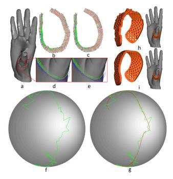
**Figure 20:** (a) Curve on a mesh. Directly using the underlying mesh normal produces local frames with jitter (b,d). The normal trace onto the unit sphere reveals this (f, green). This leads to nonsmooth synthesis results (h). We smooth the normal trace on the sphere by fitting a cubic spline (g, red), and use this to form new local frames (c,e) which are smooth and approximate the initial frames. This greatly improves synthesis results (i).
