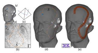
**Figure 19:** (a) The user selects points on the surface which are mapped into the parameterization domain  $\Gamma$  of  $\Psi$ . (b) A planar spline  $\hat{S}$  is constructed on  $\Gamma$ . (c) We sample a sequence of points on  $\hat{S}$ : uniformly spread arc points (blue) and all the intersection points with the mesh (red). (d) Mapping back these points onto  $\Psi$ , we form a 3D band S along which synthesis is performed (e).
