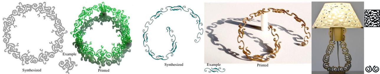
**Figure 1:** We use vector shapes as inputs to synthesize patterns along curves. The resulting patterns have a constrained topology allowing them to be 3D printed as a single piece. Left: Pattern along a circle and its printout. After printing, the pattern is a single connected object. Middle: Pattern along a curve and its printout. Right: A printed lamp modeled with our system, the shade and the foot are synthesized.
