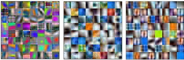
Fig. 11: First convolutional filters of the PhilippNet learned with surrogate classes (left), 10K Rome classes (middle) and 100K Rome classes. Best viewed in color.
