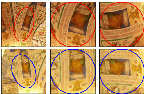
Fig. 7: Example of matching points in two different images. Salient points are extracted (left), affine rectified (middle), and normalized in rotation (right). Note that the level of invariance which remains to be covered by the patch descriptor is relatively low, as most of the work has been accomplished by the detector.
