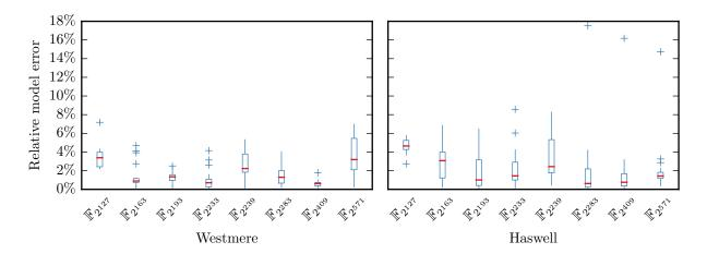
Fig. 3: Field inversion cost model relative errors (box plot). The error was calculated as the absolute value of the difference of the predicted cost and the measured cost, divided by the measured cost. The results were aggregated over all distinct optimal addition chains for all multi-square block sizes B and all values of  $c_{\text{mem}}$ . The overall median relative error was 1.50%.
