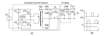
Fig. 5. Constant current source based on half-bridge converter: a) configuration; b) typical waveforms.
