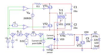
Fig. 8. PSIM model for considered constant current converter.
