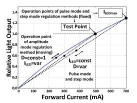
Fig. 2. Ampere-lumen curve of a common high power LED and operation points for different luminous flux regulation methods.
