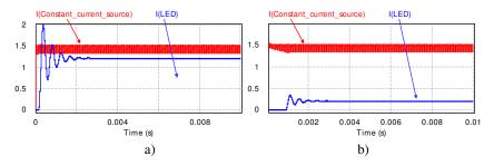
**Fig. 9.** Simulation results of the considered constant current sources operating with CF buck converter: a) startup process at 85% of maximal LED current (D=15% for CF buck); b) steady state operation at 15% of maximal LED current (D=85% for CF buck).
