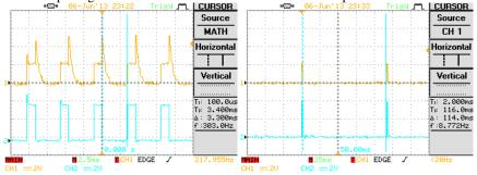
In Fig. 7 a), the time constant is the time that the voltage across LED drops from *Vcc* to *Vcc*  $\cdot e^{-1}$ , but the threshold voltage of microcontroller is around 2V. Through the proportionality rule,
