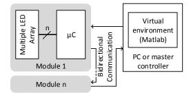
Fig. 5. Interconnection between the LED and master controller through a serial communication.
