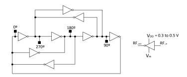
Fig. 4. Quadrature four-stage ring oscillator.
