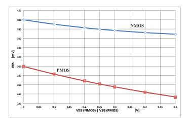
Fig. 3.  $V_{\text{th}}$  reduction for the NMOS and the PMOS transistors.
