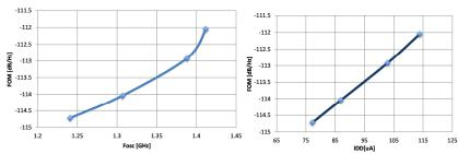
Fig. 7. FoM versus oscillation frequency
