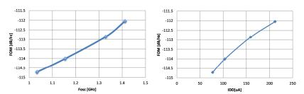
Fig. 9.FoM versus oscillation frequency.
