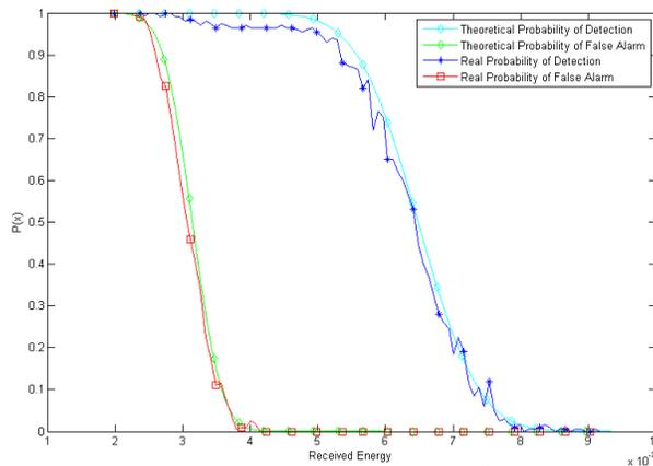
Fig. 8. Theoretical and Real Probabilities ( $T_S^{SU} = 0.0512s$ ).
