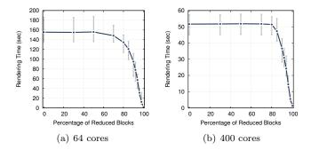
Figure 8: Run time of the rendering pipeline (average, minimum, and maximum across 10 iterations) as a function of the percentage of blocks being reduced.
