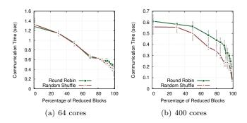
Figure 9: Run time of the redistribution component (average, minimum, and maximum across 10 iterations) as a function of the percentage of blocks being reduced.
