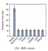
Figure 6: Run time of the rendering pipeline when none of the blocks are reduced, but load-redistribution is enabled based on scores provided by different metrics. NONE represent the case where the load has not been redistributed, SHUFFLE corresponds to random shuffling, and all others correspond to a round-robin distribution according to scores.
