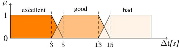
Fig. 3: Diagrammatic representation of  $\Delta t$ .
