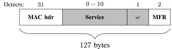
Fig. 4: Frame format with *Service* and *Service confidence*.
