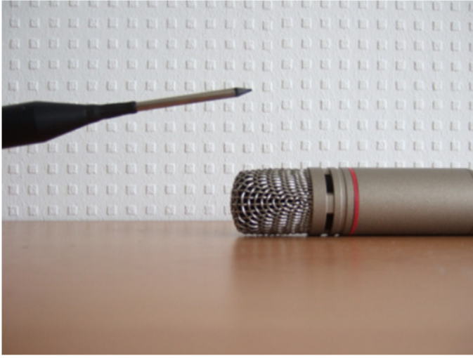
FIG. 9: Experimental protocol for audio/EM synchronization: an EM pointer hits the surface of a microphone.
