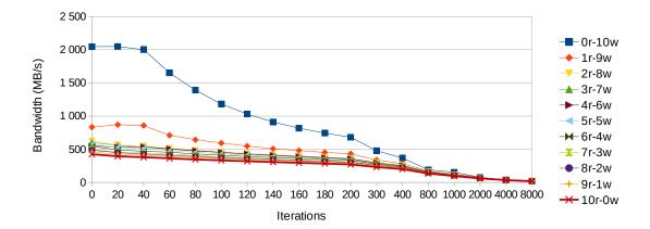
Figure 5: Bandwidth of the microbenchmark run in isolation
