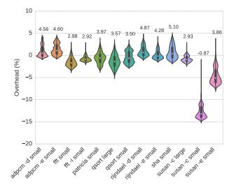
Figure 8: Overhead for MiBench applications with constant loads
