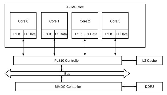
Figure 1: Architecture of the SABRE Lite board
