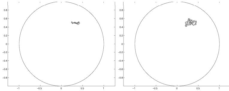
**Figure 4.** Negative isovales of the topological gradient. Noise: 5% (left) and 20% (right). (courtesy S.Amstutz, I.Horchani).
