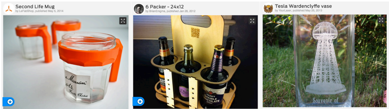
Figure 1: Things include: a) 3D designs for fabrication (3D-printed mug handle, Thing 310961, by LeFabShop); b) 2D designs for fabrication (laser-cut 6-pack holder, Thing 16643 by BrianEnigma); c) 2D designs for etching (etching on a glass vase, Thing 93972 by YourLaser, illustration by Leo Blanchette).
