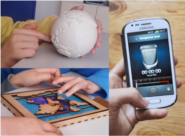
Figure 4: Top left: Probe 1, TactiGlobe, a tactile 3D printed globe. Bottom left: Probe 2, WoodMap, an interactive map with a laser-cutted overlay, using ludic audio cues. Right: Probe 3, SoundRec, an audio-recorder Android app.
