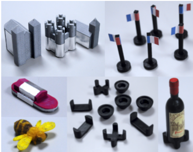
Figure 7: MapSense's Do-It-Yourself tangibles were 3D printed. Some were added sticky aluminium to be conductive. The flags were printed using conductive PLA. The bee is used with the versatile conductive supports, that can be used with any toys or objects. The bowls can be filled with scented oils or food.
