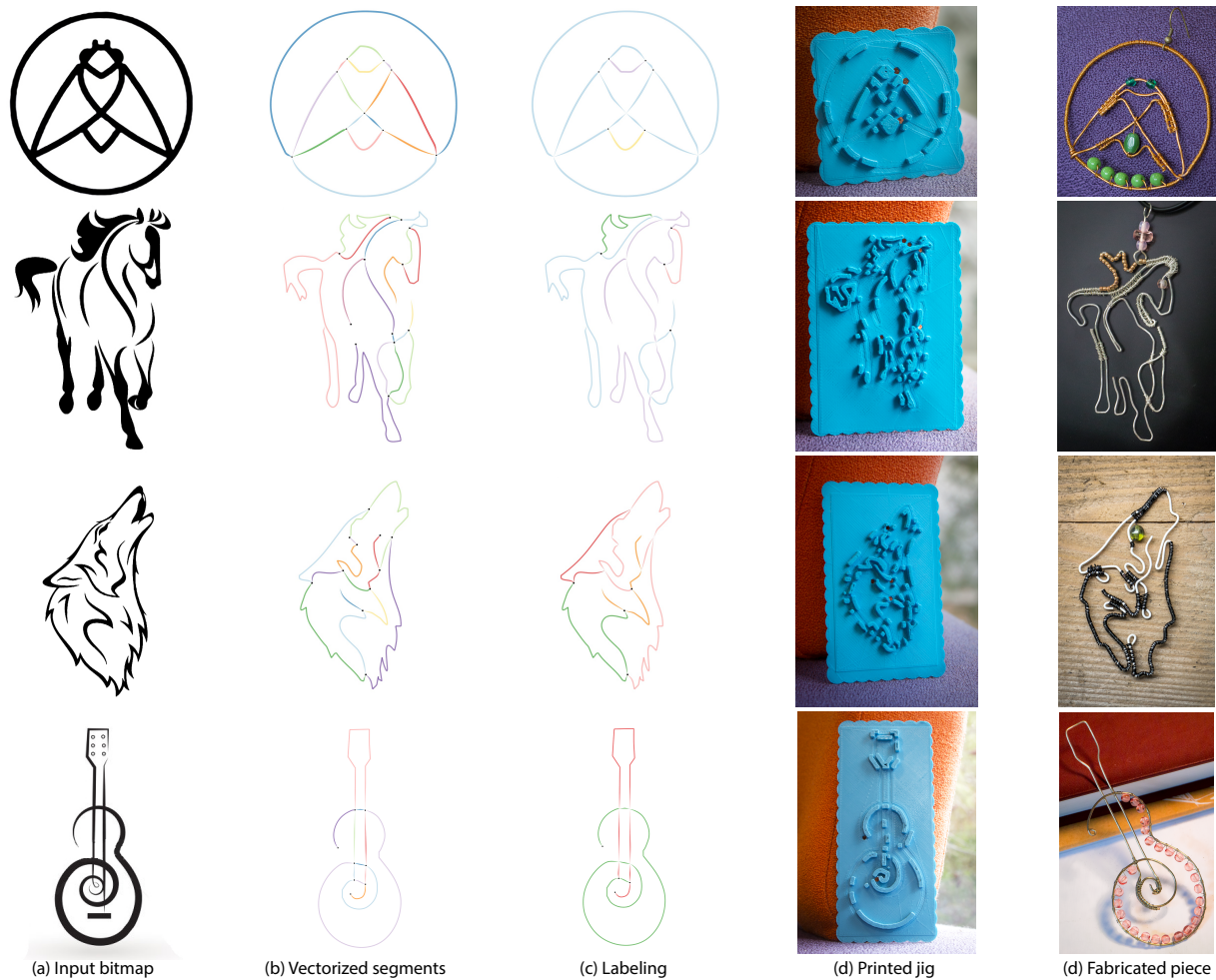
Figure 8: Clipart repositories provide a wide source of inputs for our approach. Note how our algorithm finds decompositions with few yet smooth and robust wires, such as the body of the bee and the legs of the horse.
