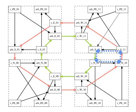
Figure 6: Illustration of the two circular paths that a packet can reach any node and the livelock loop  $r_N_10 \rightarrow arb_N_10 \rightarrow r_S_11 \rightarrow arb_S_11 \rightarrow r_N_10$ .
