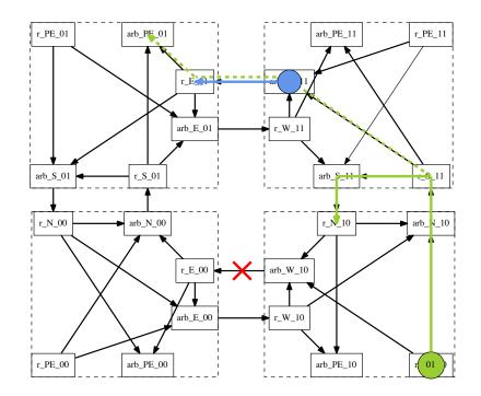
Figure 4: Illustration of the problem with the abstract model. The crossed link indicates that link from node 10 to node 00 is faulty. Solid thick arrows end in the routers handling packets. The dashed arrow indicates the route for the packet from node 10 to node 01, taken into account the failed link.
