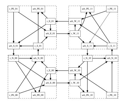
Figure 3: Architecture of the four routing nodes in a two-by-two mesh.
