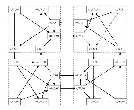
Figure 8: Improved two-by-two NoC architecture with livelock removal. Note that the modifications to avoid livelock have led to the removal of four connections that are no longer needed (i.e., between r\_S\_01 and arb\_S\_01, r\_W\_11 and arb\_W\_11, r\_S\_11 and arb\_S\_11, and r\_N\_10 and arb\_N\_10).
