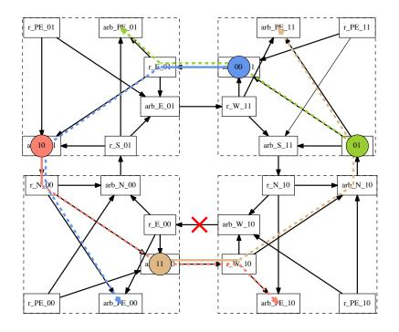
Figure 2: Illustration of a deadlock caused by a cyclic communication dependency. Each packet is represented by a circle containing its destination. A solid line coming out of a packet indicates the router where it is currently traveling to. A dashed line indicates the remaining route of a packet. The crossed link indicates that the link from node 10 to node 00 is faulty.
