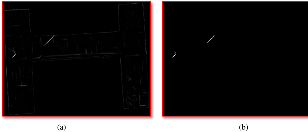
Figure 16. Example of optimized filtering, obtained in less than 4 seconds. (a) shows areas with visual impact on the links without edges and (b) is the result of threshold of these areas above half the maximum intensity.
