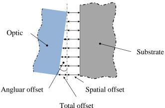
Figure 1: Model for compensation of shrinkage effects
