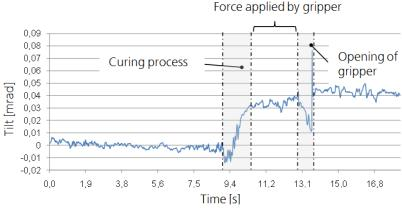
Figure 4: Tilt measurement sample of curing process
