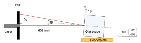
Figure 3: Principle measurement setup for shrinkage quantification
