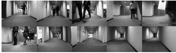
Fig. 13. Changes in the navigation environment from the mapped one: people passing by, opening of the doors, change in the local illumination due to a dead bulb and blur in the image.
