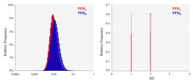
Figure 8.Input Parameters Distributions and Target SIL Distribution obtained by Monte Carlo Simulation
