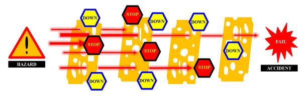
Figure 4. Independent Protection Layers against Accident
