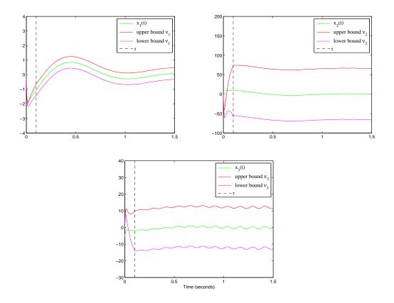
Figure 6: Example 2 with  $\tau = 0.1s$ ,  $u(t) = (2t+1)\sin(50t)$ ,  $\overline{\epsilon}_1 = 0.001$  and  $\overline{\epsilon}_2 = 0.02$
