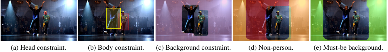
Figure 3: Constraints (see Section 3.4) used in our model for multi-person segmentation. In this setup we are provided head detections, from which we derive body boxes. We require 75% of pixels inside head detections (a) and 50% of pixels inside body boxes (b) to belong to the instance. Part (c) illustrates the background constraint (96% of this surface should be background); non-person constraints which enforce superpixels far from the person to be assigned to the corresponding label (d); and the superpixels which can only be background (e).
