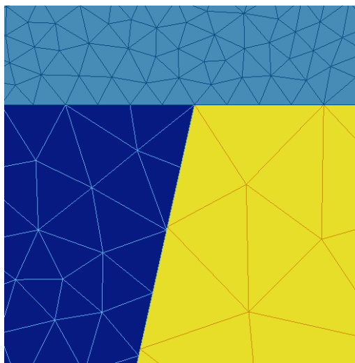
Figure 18: Illustration of the non-conforming mesh used in the case of a three layers simulation including the shore line region, zooming in on the point on which the coupling boundaries intersect.
