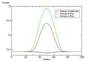
FIG. 7.4. Two dimensional test problem of laser-matter interaction taking to account the inverse Bremsstrahlung effect. Temperature, density  $\rho$  and entropy are computed at the initial time, at times 25 ps, 50 ps by the relaxation scheme proposed in this work. Temperature is scaled at its the initial value  $T_{e_0} = 2.3 \times 10^7$  K while density is scaled at  $n_{e_0}m_i/Z = 10^{27}m_i/4$  where  $m_i$  is the ion mass.
