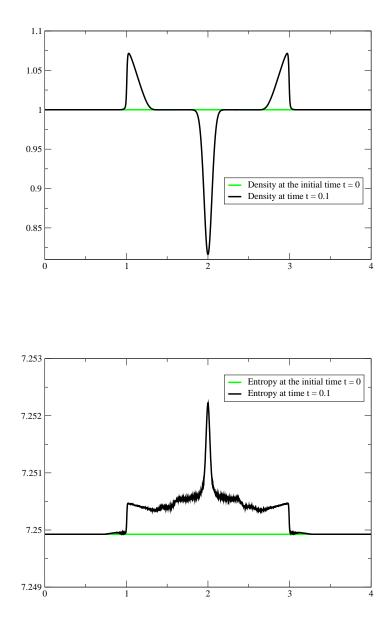
FIG. 7.1. Uniform plasma state with a gaussian-type source term: density  $\rho$  calculated at time 0.1, and entropy s computed at times 0 and 0.1 by the relaxation scheme proposed in this work.
