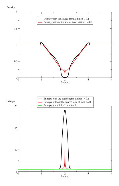
FIG. 7.2. Two rarefaction waves problem with and without a gaussian-type source term: density  $\rho$  computed at time 0.05, and entropy s computed at times 0 and 0.1 by the relaxation scheme proposed in this work.
