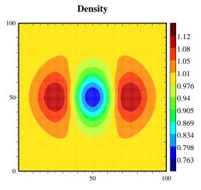
FIG. 7.5. Two dimensional test problem of laser-matter interaction taking to account the inverse bremsstrahlung effect. Temperature, density  $\rho$  and entropy are computed at 50 ps by the relaxation scheme proposed in this work. Temperature is scaled at its the initial value  $T_{e_0} = 2.3 \times 10^7$  K while density is scaled at  $n_{e_0}m_i/Z = 10^{27}m_i/4$  where  $m_i$  is the ion mass.
