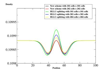
FIG. 7.3. Two dimensional test problem of laser-matter interaction: density  $\rho$  computed at time 5 ps by the relaxation scheme proposed in this work. The comparisons are also proposed with the solutions rendered by the HLLC-splitting scheme.
