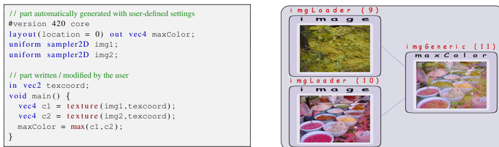
Figure 6. Left: The header of the fragment shader is automatically generated depending on user settings (inputs, outputs, parameters, etc). The main function might be directly modified to obtain the desired effect. The maximum color is displayed here, as shown on the right.
