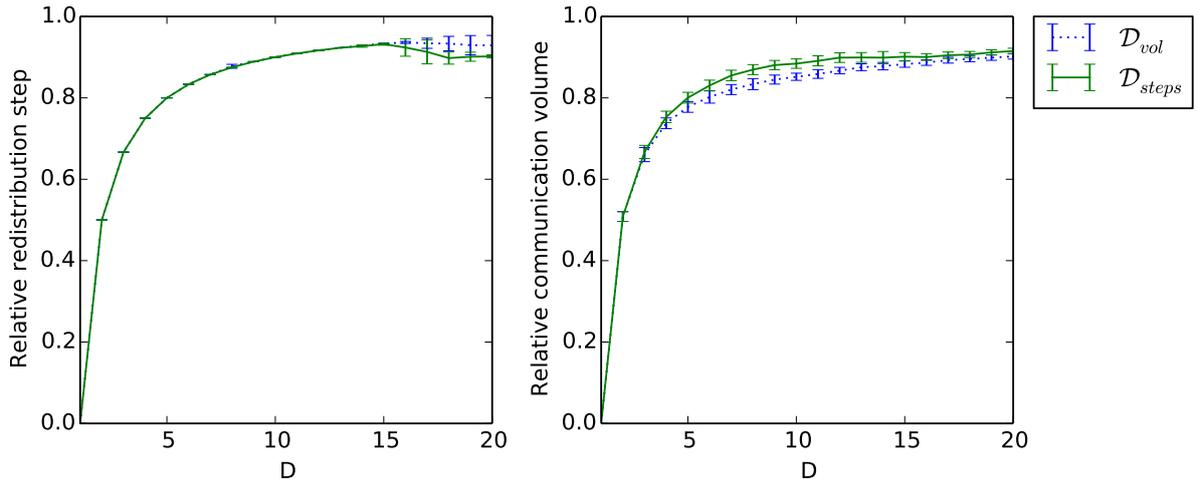
Figure 2: Performance of  $\mathcal{D}_{vol}$  (computed by Algorithm 1) and  $\mathcal{D}_{steps}$  (computed by Algorithm 2) relatively to the canonical distribution, for a random initial distribution and for both metrics.
