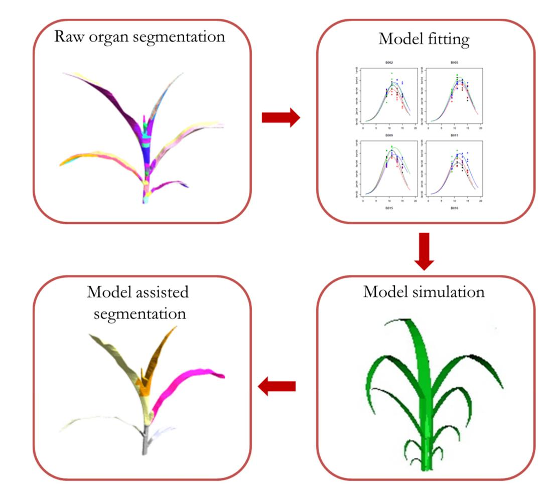
Multi-view plant images from PhenoArch are binarised and used to reconstruct plants in 3D. The 3D skeleton is extracted and separated into stem (central vertical skeleton elements) and leaves. 3D voxels are segmented by propagating skeleton segmentation.
