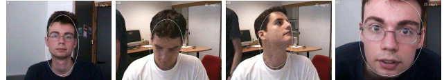
Figure 1: Example of face tracking. First and second moments provides an ellipse which delimit the face in the image
