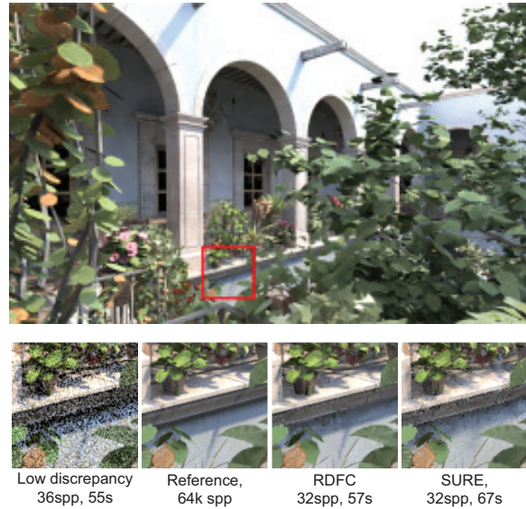
Figure 12: Equal-time comparison of Rousselle et al. [RMZ13] (RDFC, main image) and Li et al. [LWC12] (SURE, in close-ups). RDFC is more robust to noisy error estimates, and it includes a feature to capture soft shadows from direct illumination, which leads to significant quality improvements.
