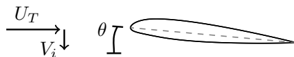
Figure 19: Scheme of operating conditions at a blade section: the uncertain variables are the pitch angle \theta and the induced velocity V_i . The velocity component U_T is the velocity tangential to the rotor disk.
