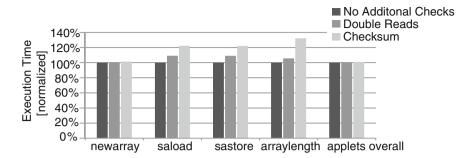
Fig. 5. Graphical representation of the performance impact of the additional double read and checksum calculations for selected bytecodes and the overall time of the measured applets.
