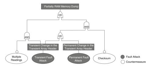
Fig. 2. Fault tree overview of the different possible attack paths to fulfill a partial memory dump of the RAM by a fault attack. Furthermore, effective countermeasures against the two general types of fault attacks are listed.
