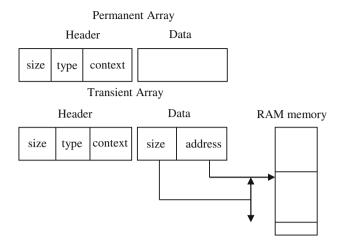
Fig. 1. Structure of transient and permanent arrays.
