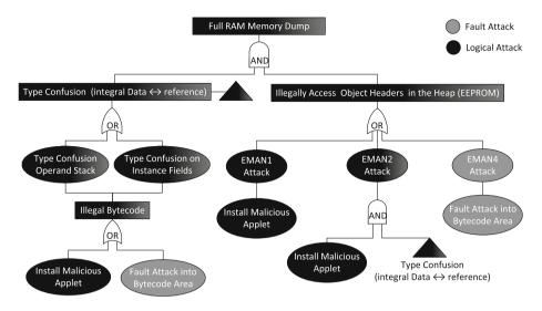
Fig. 3. Fault tree overview of the different possible attack paths and needed attack preconditions to fulfill the memory dump attack of this work.
