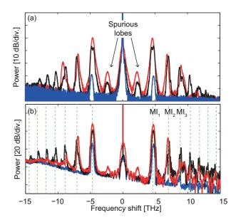
FIG. 7. (Color online) Spectra recorded at the output of fibers A, B and C (we use the same color label than in Fig. 5): (a) Experiments; (b) Numerical simulations which include higher-order dispersions  $\beta_3 = 5.6 \times 10^{-41} \text{ s}^3/\text{m}$ ,  $\beta_4 = -1 \times 10^{-55} \text{ s}^4/\text{m}$  and losses  $\alpha = 5 \text{ dB/km}$ .
