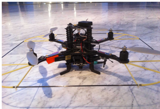
Figure 32: AscTec Pelican quadcopter [55] equipped with a monocular camera.
