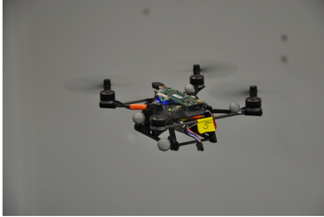
Figure 23: Our nano quadrotor from KMeI Robotics: a 150g and 18cm sized platform equipped with an integrated Gumstix Overo board and MatrixVision VGA camera.
