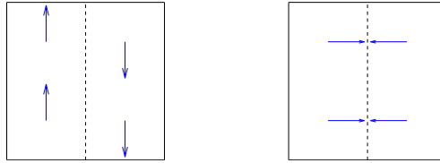
FIGURE 8. Sketch of shear velocity (a) and collisional velocity (b).
