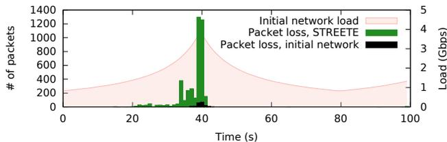
Fig. 10: Packet loss.
