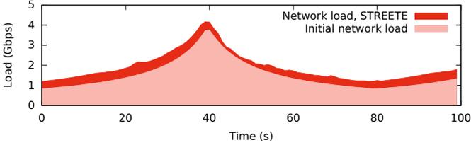
Fig. 8: Generated load and overhead of STREETE.
